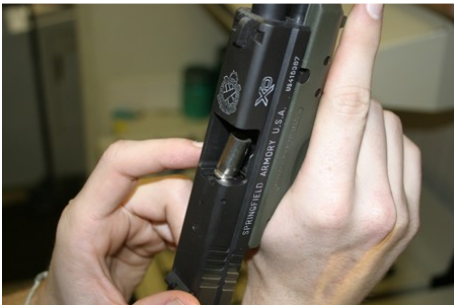
Set the cartridge behind the extractor, just sitting on top of the ejector.
