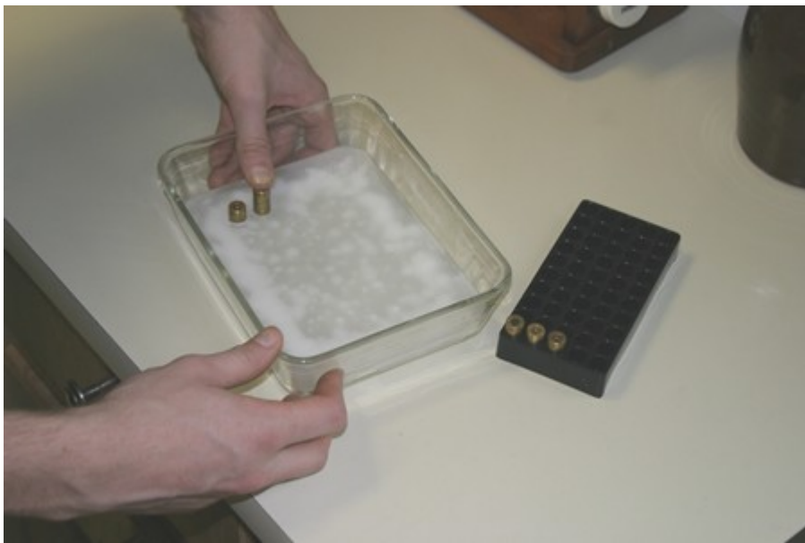
Be careful to press the brass in squarely in order to get a good bullet.
