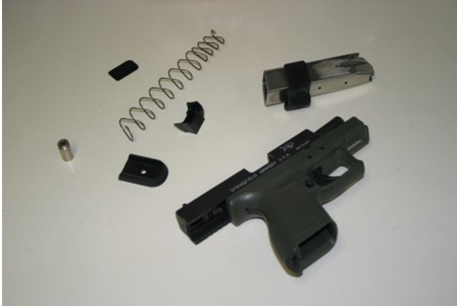
Remove the guts from a magazine. Put the floor plate back on the magazine, and insert into the gun. You won't need the spring or follower.
