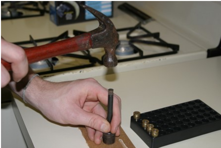
A good solid smack with a hammer and the primer comes right out.
